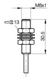
**Inductive Sensors** BES 516-324-SA 17-05 M8x1 x 30.5 normally-open Sn=1,2mm shielded pressure rated to 10 bar
